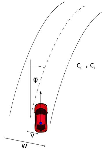
Fig. 3: Road model for video-based lane recognition including the parameter lane width ( $w$ ), relative yaw angle ( $\varphi$ ), vertical offset ( $v$ ) from the middle of the lane and two curvature parameter ( $c_0, c_1$ ).
