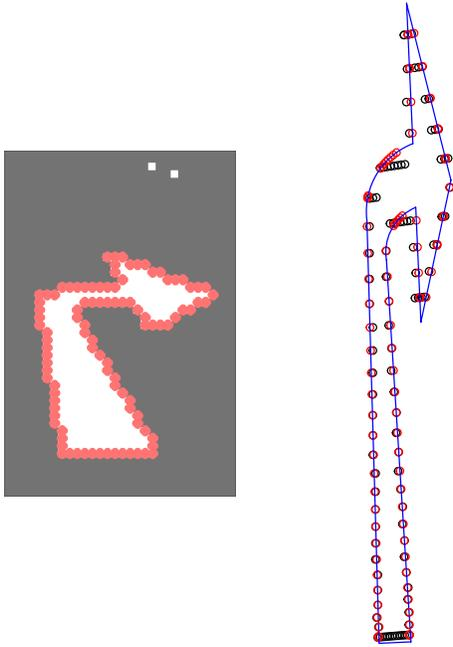
Fig. 10: The left figure shows the extracted pixel list of the connected component. The black points on the right figure indicate the pixel list reprojected to the street plane. The red ones are the perpendicular points on the prototype.
