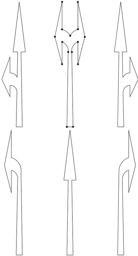
Fig. 5: Arc spline models of the arrow markings (ahead-left, left-right, ahead-right, left, ahead, right). In the middle image of the first row the breakpoints of the arc spline are accentuated.
