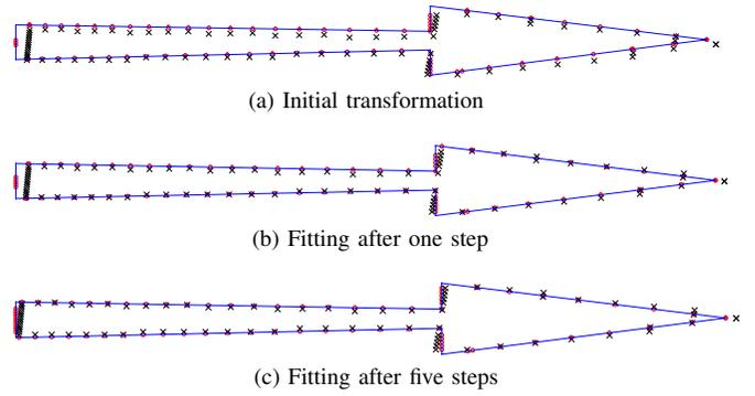
Fig. 6: Iterations of prototype fitting. The higher the number of iterations the smaller are the transformation changes. Prototype fitting converges to a stable state.
