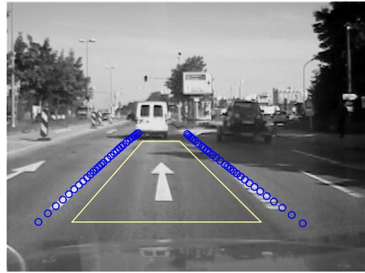
Fig. 2: The drivable area in front of the vehicle as a result of lane recognition system.
