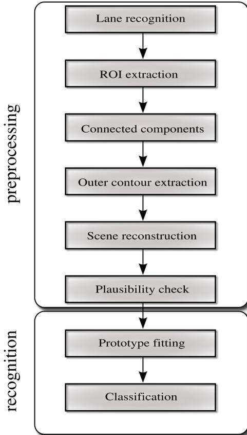
Fig. 1: Overview of the processing chain
