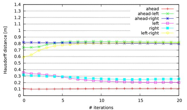
Fig. 8: Hausdorff distance as a function of the number of iterations for all arrow prototypes.
