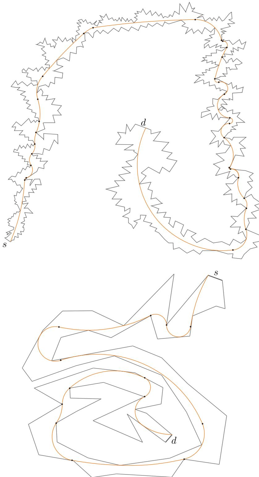
Figure 79: Example of two start-destination channels given by simple polygons and corresponding continuous smooth arc paths. Top: 1047 vertices; 29 segments; Bottom: 61 vertices; 17 segments;
